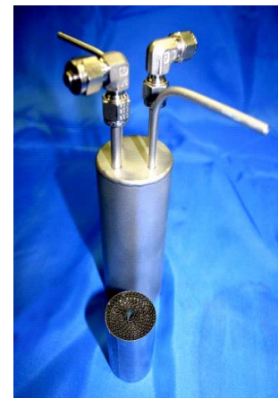
Figure 2: compact hydrogen generation using monolithic catalyst structures
