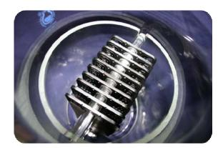
Ex-situ accelerated ageing  $(H_2SO_4 @ 80^{\circ}C \text{ or } H_3PO_4 \text{ c}=85\% @ 180^{\circ}C)$
